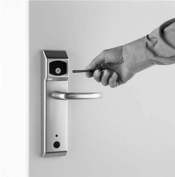
Figure 13.25 Offline terminal integrated into a doorplate. The lock is released by holding the authorized transponder in front of it. The door can then be opened by operating the handle. The door terminal can be operated for a year with four 1.5 V Mignon batteries and even has a real time clock that allows it to check the period of validity of the programmed data carrier. The terminals themselves are programmed by an infrared data transmission using a portable infrared reader (reproduced by permission of Häfele GmbH, D-Nagold)
