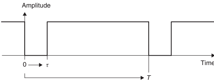
Figure 6.8 Representation of the period duration T and the bit duration \tau of a binary code signal
