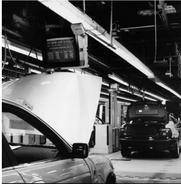
Figure 13.59 After successful identification of the vehicle, its specific data is interrogated and displayed (reproduced by permission of Pepperl & Fuchs GmbH, Mannheim)
