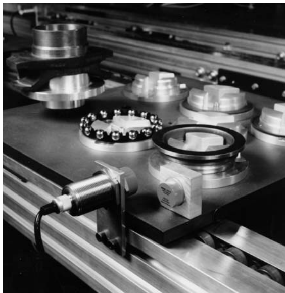
Figure 13.60 Individual components of a clutch release stop on a revolving pallet. Transponder and reader antenna are visible in the lower part of the photo (reproduced by permission of Pepperl & Fuchs GmbH, Mannheim)
