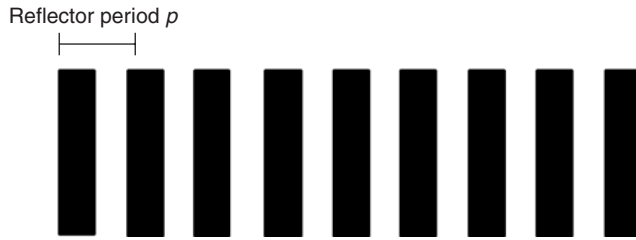
Figure 4.96 Geometry of a simple reflector for surface waves (reproduced by permission of Siemens AG, ZT KM, Munich)
