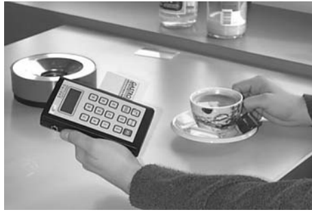
Figure 11.28 Reader for portable use in payment transactions or for service purposes (photo: LEGIC® reader reproduced by permission of Kaba Security Locking Systems AG, CH-Wetzikon)
