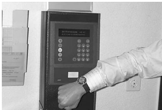
Figure 13.24 Access control and time keeping are combined in a single terminal. The watch with an integral transponder performs the function of a contactless data carrier (reproduced by permission of Legic®-Installation, Kaba Security Locking Systems AG, CH-Wetzikon)
