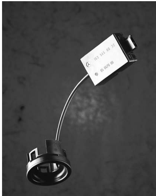
Figure 13.43 The antenna of the electronic immobilisation system is integrated directly into the ignition lock (reproduced by permission of Deister Elektronik, Barsinghausen)
