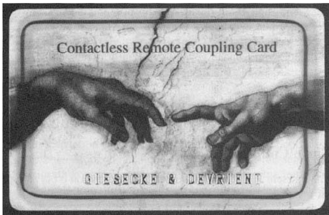
Figure 2.12 Semitransparent contactless smart card. The transponder antenna can be clearly seen along the edge of the card (reproduced by permission of Giesecke & Devrient, Munich)
