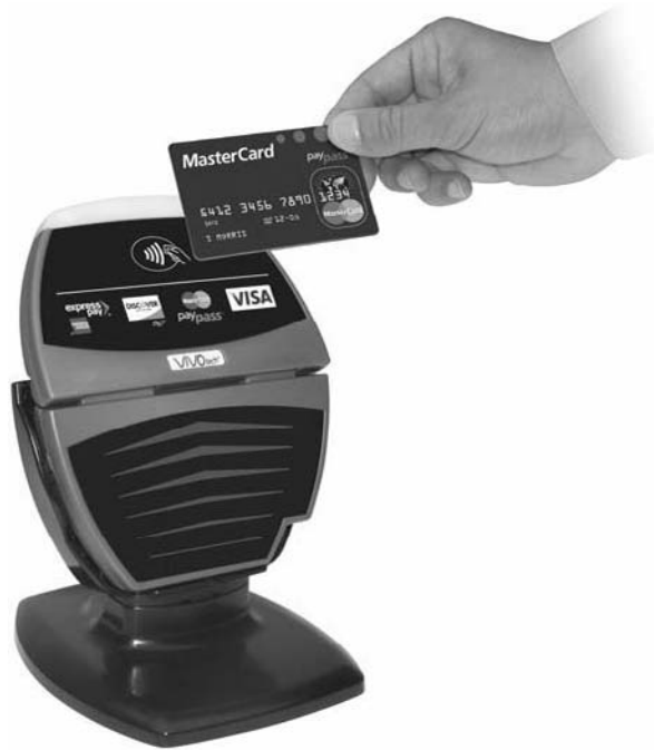
Figure 13.10 Payment process with a contactless smart card at a contactless POS terminal (reproduced by permission of Vivotech)
