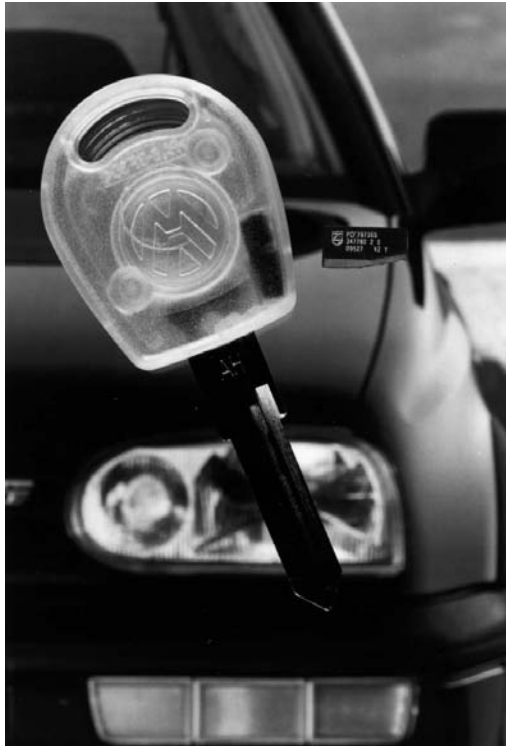
Figure 13.42 Ignition key with integral transponder (reproduced by permission of Philips Electronics N.V)
