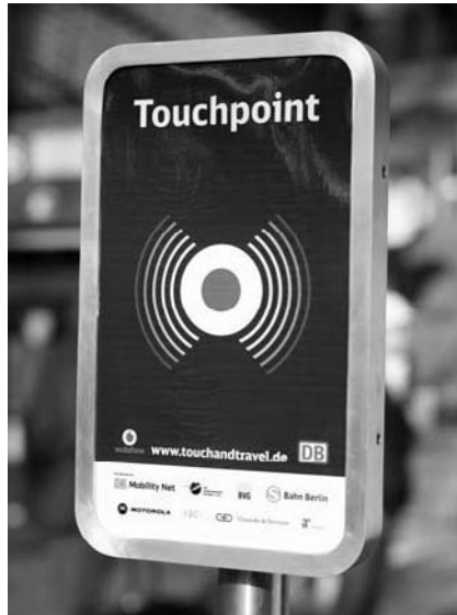
Figure 13.16 The touchpoint only has a passive transponder that can be read out by an NFC-enabled mobile phone (reproduced by permission of Deutsche Bahn)
