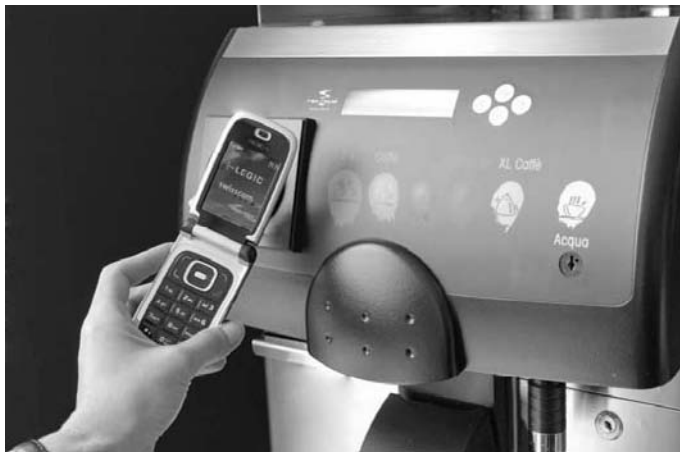
Figure 13.17 An NFC-enabled mobile phone with the corresponding payment application simulates a contactless credit or debit card (reproduced by permission of LEGIC Ident systems AG, CH-Wetzikon)
