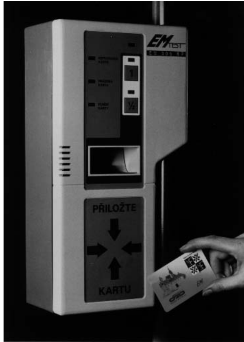
Figure 13.1 Contactless reader in a public transport system (photo: Frydek-Mistek project, Czechoslovakia, reproduced by permission of Philips Semiconductors Gratkorn, A-Gratkorn)
