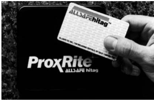
Figure 1.7 RFID reader and contactless smart card in practical use (reproduced by permission of Kaba Benzing GmbH)
