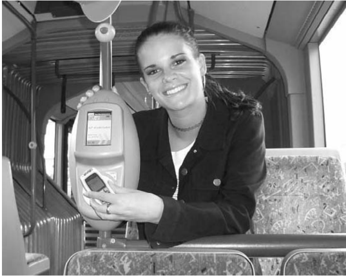
Figure 13.13 The electronic public transportation ticket get >> in, which allows customers to check in and out of busses using their mobile phones and NFC technology (reproduced by permission of © RMV)
